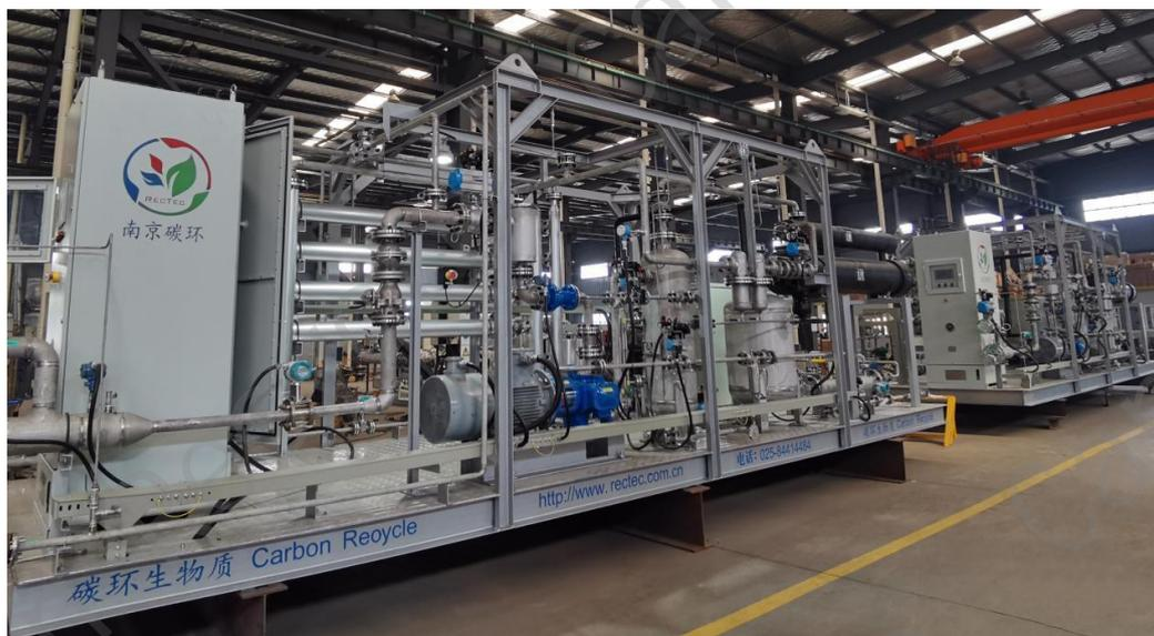
Fig. 11: Photo of 200Nm<sup>3</sup>/h N-hexane recovery equipment on site
